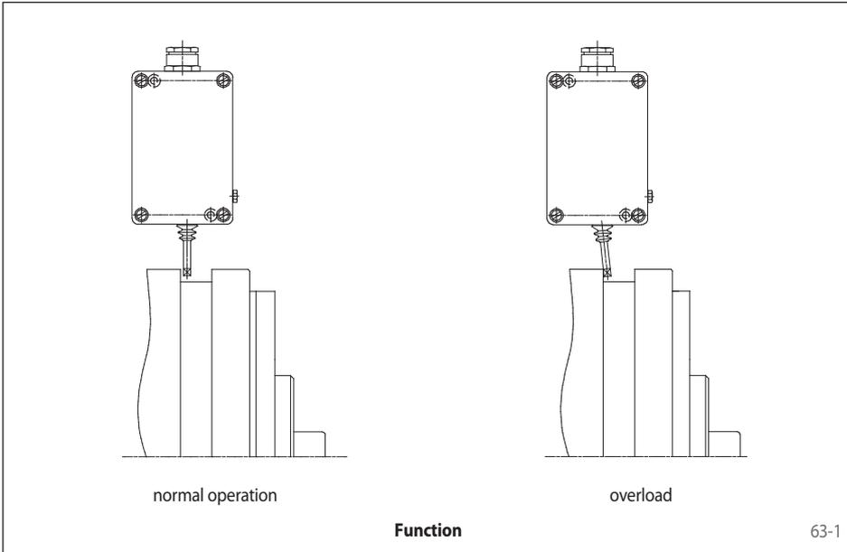
It is possible with SIKUMAT® Torque Limiters to utilise the axial movement during an overload occurrence to actuate a proximity switch so that when the preset limit torque is exceeded, the drive can be switched off electrically and/or a signal can be triggered.
